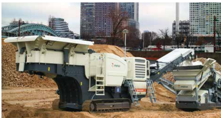
TOP: German research organisation the Fraunhofer Institute has launched a project to recycle the five million metric tonnes of building rubble produced in the country each year ABOVE: Metso's track-mounted Lokotrack LT106 crushing plant is used for recycling applications
